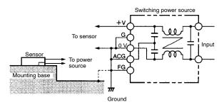
Insert a plastic insulator about 10 mm thick between the sensor and the mounting.
